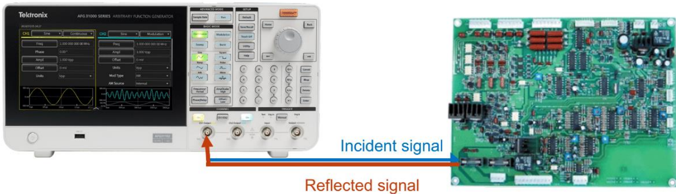
Fig. 2. InstaView real-time waveform monitoring. Due to impedance mismatches between the AFG and the DUT, the output waveform from the AFG can be different from what is observed at the DUT. So typically an oscilloscope is needed to check the signal at the DUT. However, the AFG uses the reflected signal to recreate the waveform seen at the DUT, eliminating the need for the external scope.
