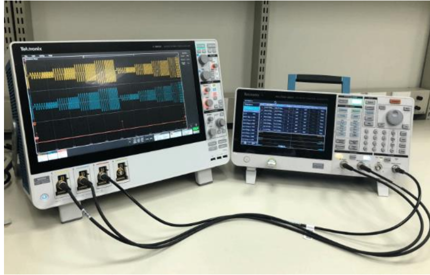
Fig. 3. An integrated waveform sequencer reduces the cost of generating complex waveforms with complex timing. Like an MP3 player, the AFG31000 can output waveforms in a user defined sequence.
