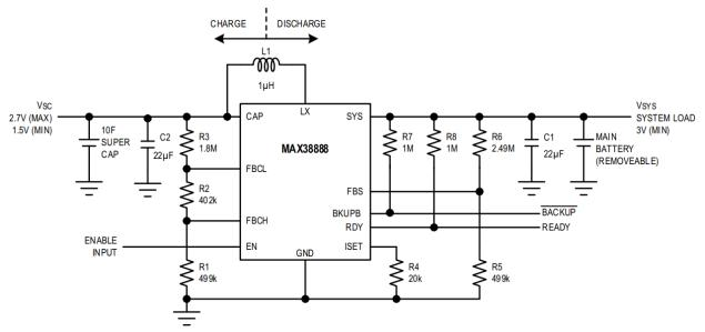
Figure. The first member of the Continua family of backup power regulators, the MAX38888 charges and discharges a backup supercapacitor or capacitor bank to deliver continuous power to critical systems when the main power is off. It operates with up to 95% efficiency during charge and discharge operations.
