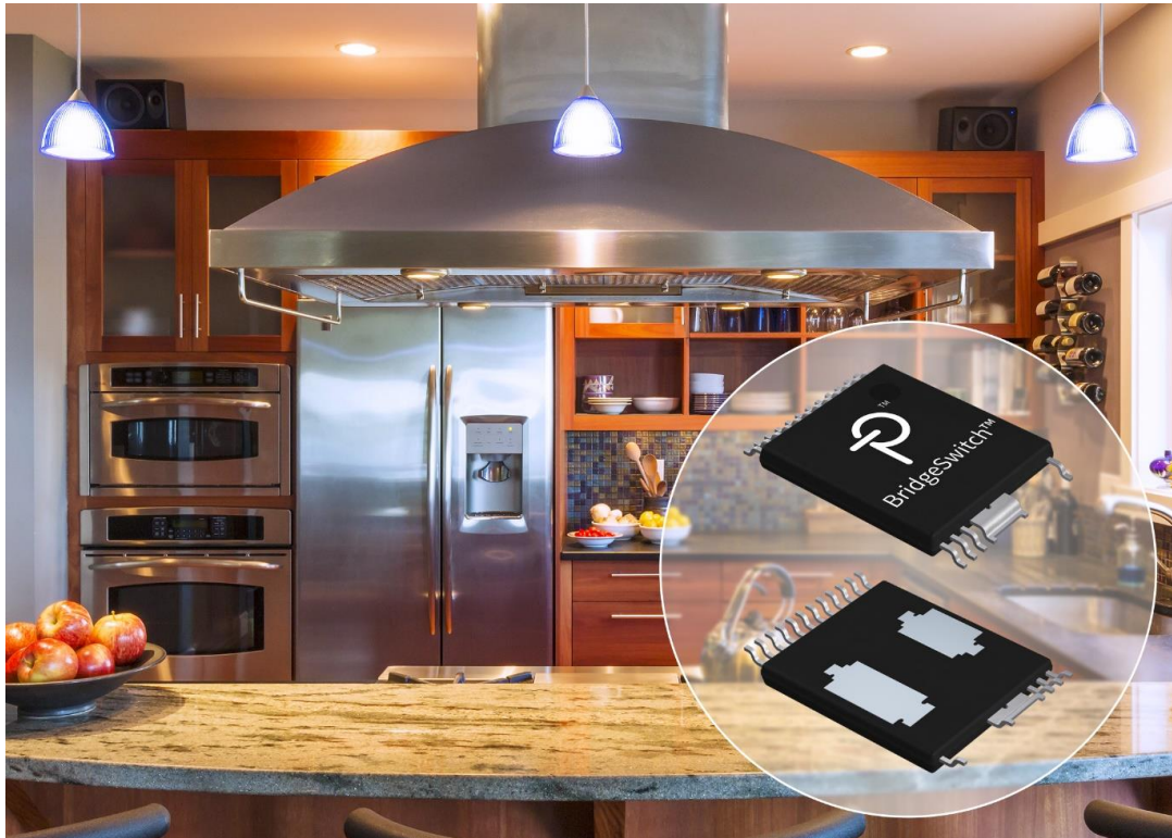
Fig. 1. The BridgeSwitch family of integrated half-bridges dramatically simplifies the development and production of high-voltage inverter driven two- or three-phase PM or BLDC motor drives. It incorporates two high-voltage n-channel power FREDFETs with low- and high-side drivers in a single small-outline package. Offering inverter conversion efficiency of up to 98.5% in brushless dc (BLDC) motor drive applications up to 300 W and a distributed thermal footprint, the IHB driver eliminates the need for a heatsink.
