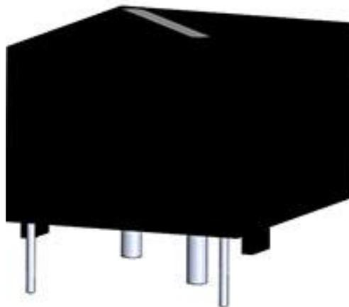
*Figure. Intended for monitoring currents in high-frequency applications such as switch-mode power supplies, LED lighting, etc., the CST25 series current sense transformers are offered with a built-in sense winding allowing for ease of use. These current sense transformers are fully encapsulated allowing for a high isolation of 4000 VAC between primary and secondary windings.*
