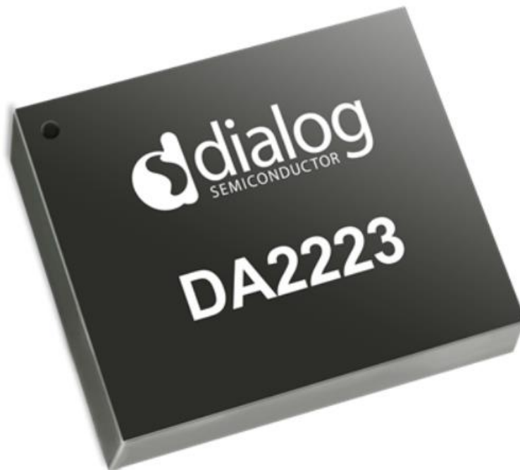
Figure. A complete WattUp wireless power receiver can be realized using a single 1.7-mm x 1.4-mm x <0.5-mm DA2223 IC coupled with a matching circuit made from two standard discrete components and a tiny 2-mm x 3-mm antenna, which itself can be formed using simple printed circuit board tracking. Such a small form factor makes it well suited for use in small electronic devices where a coil-based wireless charging system is not practical.
