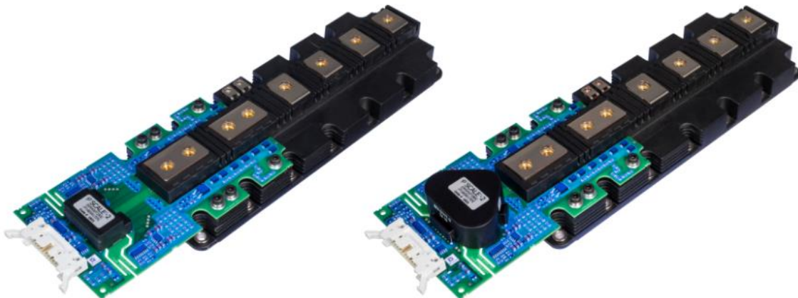
Fig. 1. The 2SP0430T2XX plug-and-play gate driver boards are designed for use with Infineon's PrimePACK3+ and Fuji-equivalent IGBT modules for two-level and three-level applications, providing reinforced isolation for 1200-V and 1700-V IGBT modules and meeting standards such as IEC60664-1, IEC61800-5-1, PD2 and PD3.
