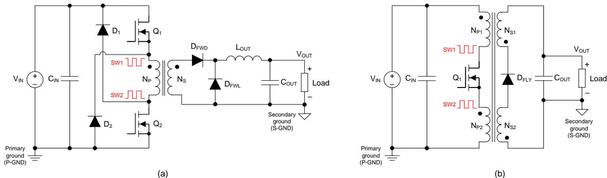
Fig. 1. Balanced-winding topologies with symmetrical primary-side circuits and equal-magnitude, out-of-phase dv/dt switching waveforms for a lower CM noise signature: two-switch forward converter (a); flyback converter with split primary and secondary windings (b).
