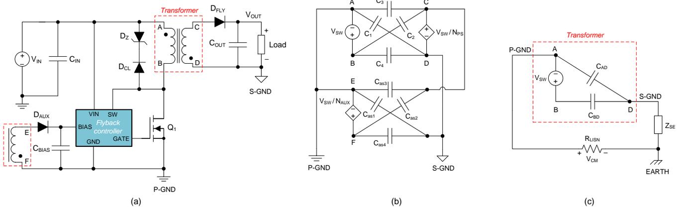
Fig. 4. Flyback converter with auxiliary winding (a), lumped CM parasitic capacitance model for a three-winding flyback transformer (b) and CM noise-equivalent circuit using a two-capacitor transformer model (c).
