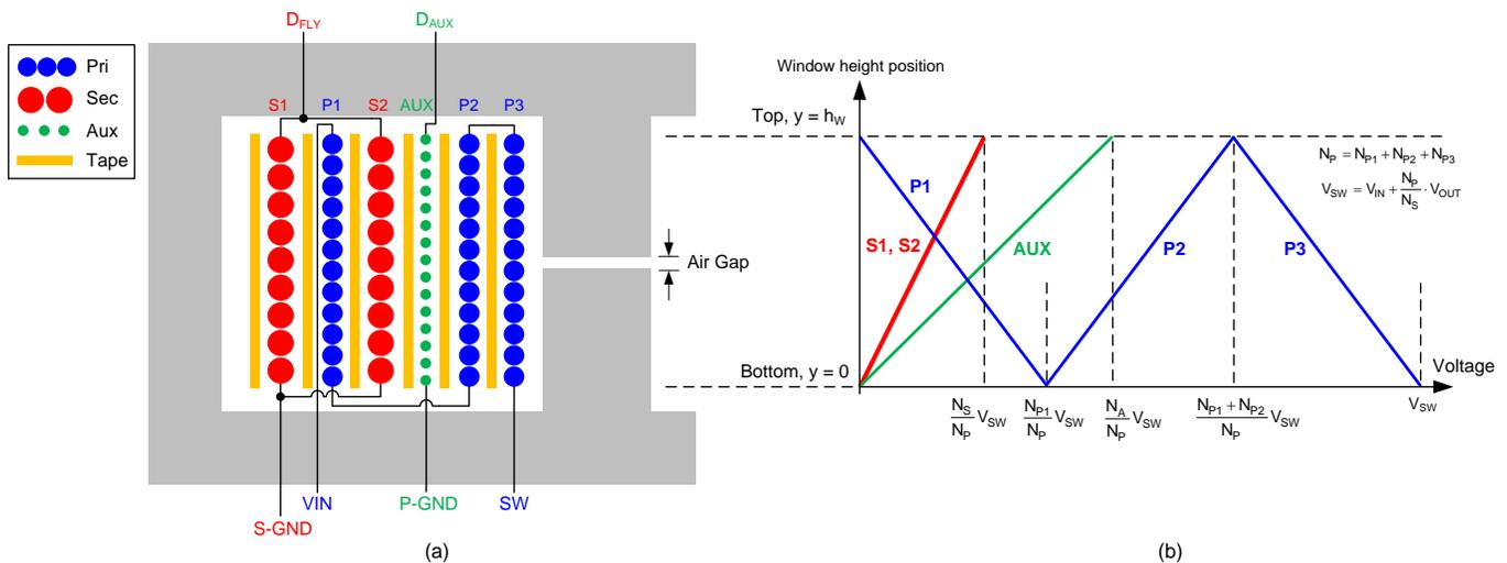
Fig. 5. Flyback transformer with a sandwiched winding layer structure (a) and voltage distributions of layers across the winding window (b).
