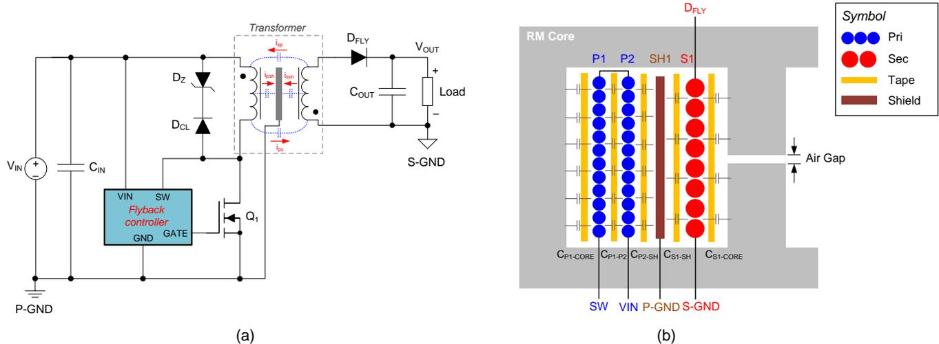
Fig. 3. Flyback converter with a conventional electrostatic foil shield winding placed between primary and secondary layers and connected to P-GND (a) and a winding layer structure of one transformer winding window (b).
