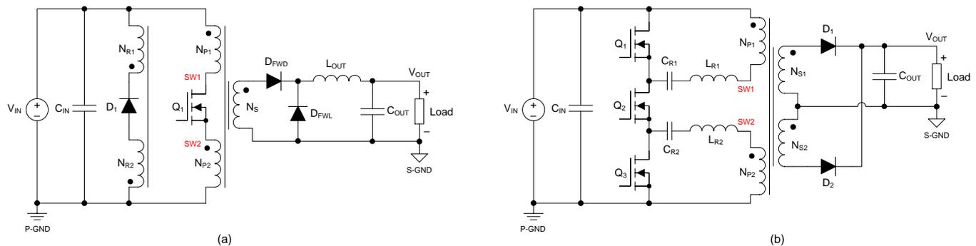
Fig. 2. Symmetrical primary winding design applied to the single-switch forward converter (a) and LLC resonant converter (b).
