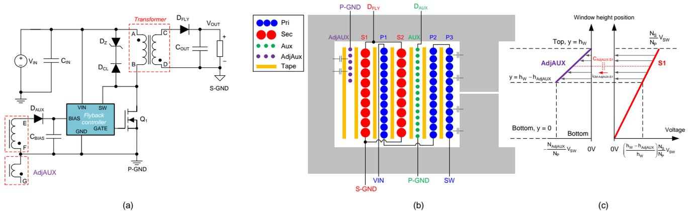
Fig. 6. Adding an adjustable auxiliary winding on the outer layer to cancel CM noise: schematic (a), winding arrangement (b) and voltage and current distributions (c).
