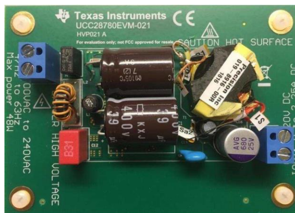
Fig. 4. 45-W ACF reference design. © 2019 How2Power. All rights reserved.
