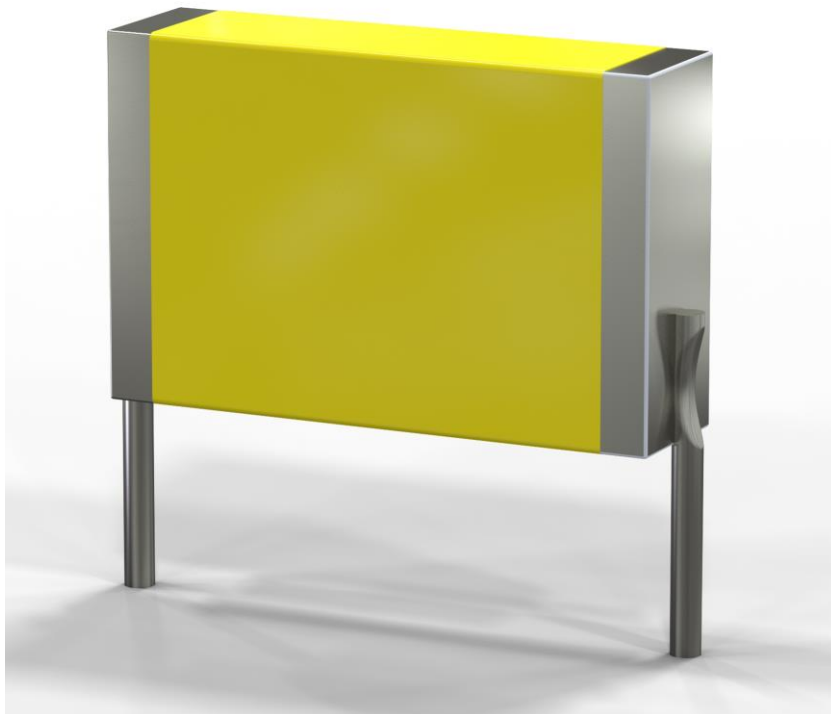
Figure. Type RA capacitors are constructed using stacked metallized polyester protected with an impregnated sealant, which eliminates the need for an external case and leads to high energy density. Available in capacitance values ranging from 0.1 \mu\text{F} to 10.0 \mu\text{F} , voltage ratings of 100, 250, 400 and 500 Vdc, these capacitors cover a broad range of applications in power electronics.
