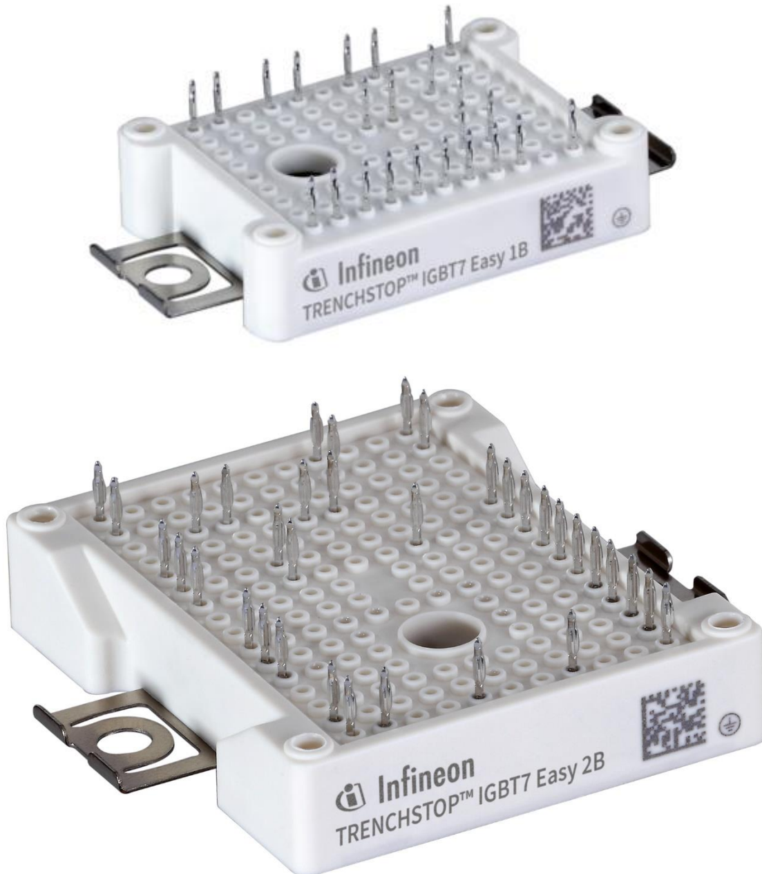
Figure. Packaged in the well-known Easy housing, the 1200-V TRENCHSTOP IGBT7 modules are designed with the same pin out as TRENCHSTOP IGBT4 modules, which eases migration from the older devices. However, the new modules enable a higher output current in the same package, or a similar output current in a smaller package. The TRENCHSTOP IGBT7 chip performs with much lower static losses than the IGBT4. Its on-state voltage is reduced by 20%.
