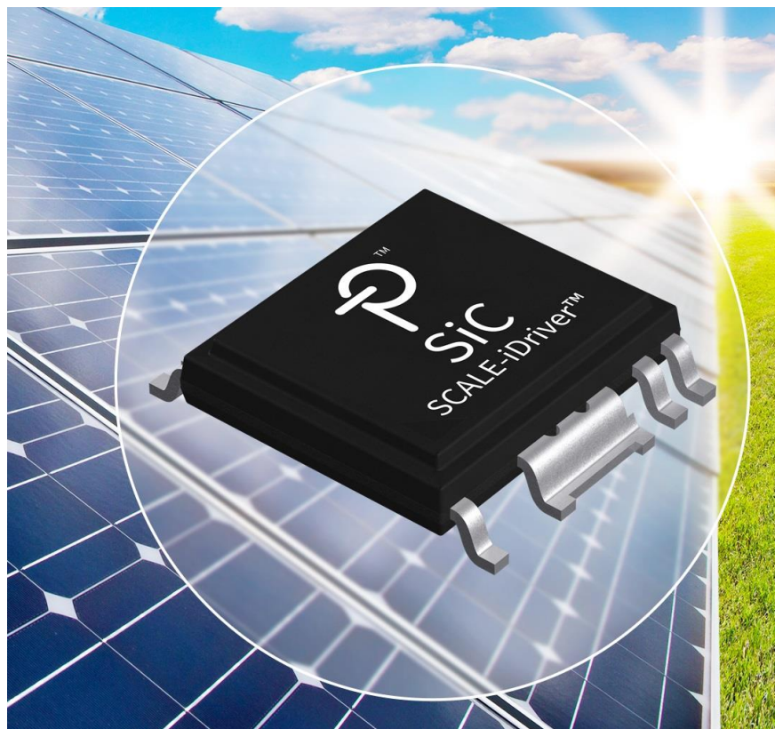
Fig. 1. Housed in an eSOP-R16B package, the SIC1182K SCALE-iDriver SiC MOSFET gate driver delivers up to 8 A at a junction temperature of 125°C, allowing it to support SiC-MOSFET inverter designs up to several hundred kilowatts without a booster stage. It also features FluxLink communications technology, which offers high reliability and reinforced galvanic isolation up to 1200 V, and protection circuits that achieve 5-μs shutdown.
