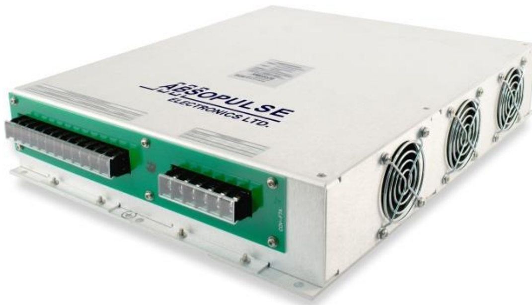
Figure. The microprocessor-controlled FCP 1K-F7W ac-ac frequency converters provide a split-phase ac-output stage for various configurations including 115-Vac split phase/60-Hz each and single-phase 115 Vac/400 Hz or 230 Vac/50 Hz. In addition, a high-voltage version which generates 400- to 450-Vac single phase is also available. The frequency converters operate from a power factor corrected universal input range of 95 to 264 Vac, 47 to 63 Hz. In addition, 400-Hz input operation is available on request.
