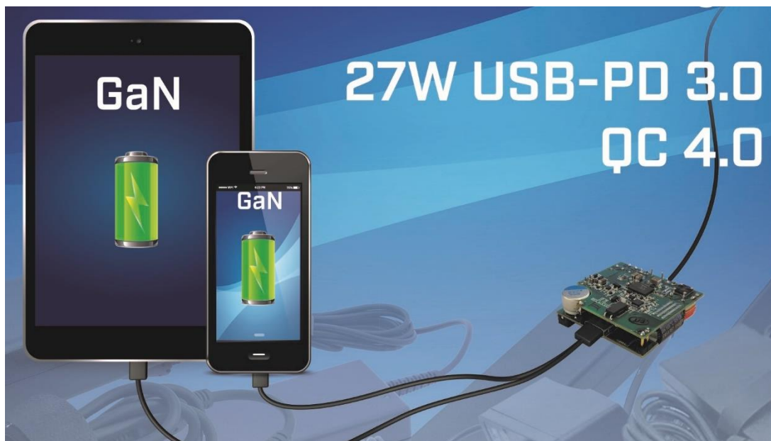
Figure. Using a Navitas' high-speed, half-bridge GaNFast power IC in the active clamp flyback (ACF) topology, the 27-W reference design measures only 39 mm x 37 mm x 16 mm (uncased) and achieves a power density of 1.2 W/cc (19 W/in 3 ) uncased and 0.7 W/cc (11 W/in 3 ) assuming a 2.5-mm case thickness.
