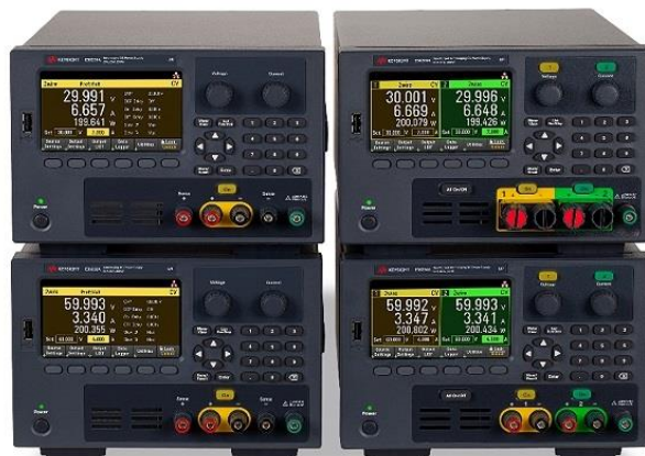
Figure. The E36200 series of single- and dual-output power supplies provide the same measurement and advance capabilities as the company's E36300 triple-output power supply series, but deliver higher current and higher voltage. These autoranging dc power supplies offer ratings of 30 V, 20 A, 200 W or 60 V, 10 A, 200 W with single output; or ratings of 30 V, 20 A, 400 W or 60 V, 10 A, 400 W with dual output.
