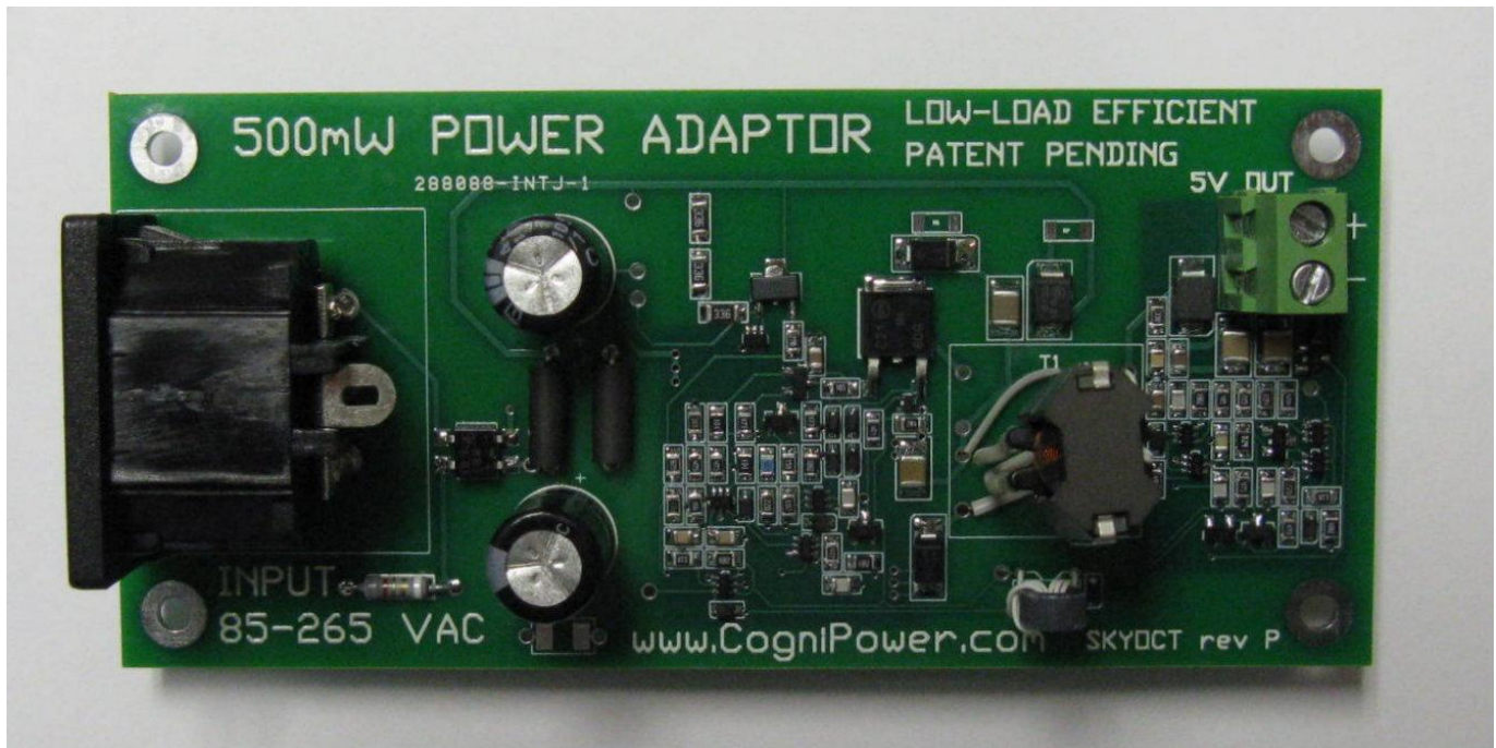
Fig. 3. Prototype DPR power converter measured at over 95% efficiency.
