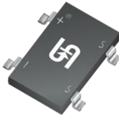
Figure. TBS series SMD bridge rectifiers optimize higher power applications and prevent arcing problems through increased creepage distance with a wider pin distance (3.6 mm) between L and N. These rectifiers have a surge current up to 150 A (8.3 ms half sine wave) and 400 A (1-ms half sine wave)—much higher than the surge current of the standard SMD bridge rectifiers on the market, according to the vendor. The product family saves manufacturing assembly costs in comparison with rectifiers in DIP packages and increases power density based on lower thermal resistance.
