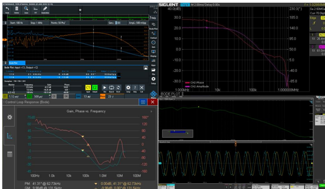
Fig. 2. The software options on the new scopes enable Bode Plot and PSRR measurements but are not sufficient on their own. To perform these control loop measurements, the stimulus signals from the oscilloscope or AWG to the power supply under test must be injected—a function performed by the Picotest injectors. While there are others offering injection transformers, according to Picotest their FRA bundle is the only commercially available solution that supports all of the listed scope manufacturers and their FRA features.
