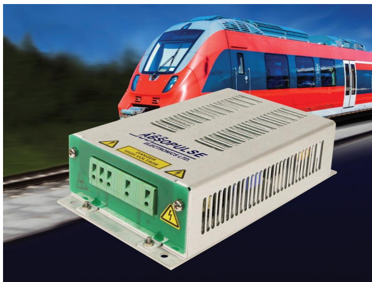
Figure. Operating from 750 V, the traction voltage required for mass transit vehicles, the HVI 41R-F1 dc-dc converter delivers a regulated 24-V/2-A output or custom output, while achieving a typical efficiency of 85% at full load. The converter is designed for up to 30 years of operating life.
