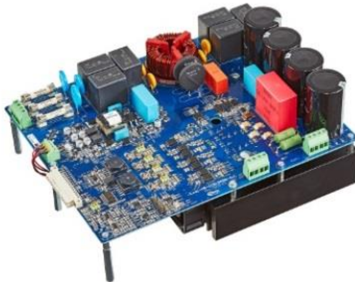
Figure. Intended to support design of industrial drives with a max of 7.5-kW motor output, the EVAL-M5-E1B1245N-SiC evaluation board combines an EasyPACK 1B with CoolSiC MOSFET, a three-phase ac connector, an EMI filter, a rectifier and a three-phase output for connecting the motor. This board was developed to help customers take their first steps in designing SiC MOSFETs in motor drives.
