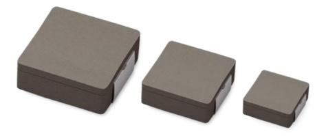
Comprising a total of 102 devices covering an inductance range from 0.10  $\mu$ H to 47.00  $\mu$ H, the METCOM series offers DCR values as low as 1.5 m $\Omega$ . The inductors can support currents up to 35.4 A and operating temperatures between -55°C and +155°C. With footprints as small as 5.3 mm x 5.00 mm and profiles as low as 2.0 mm, the METCOM series is well suited for densely-packed modern power applications.
