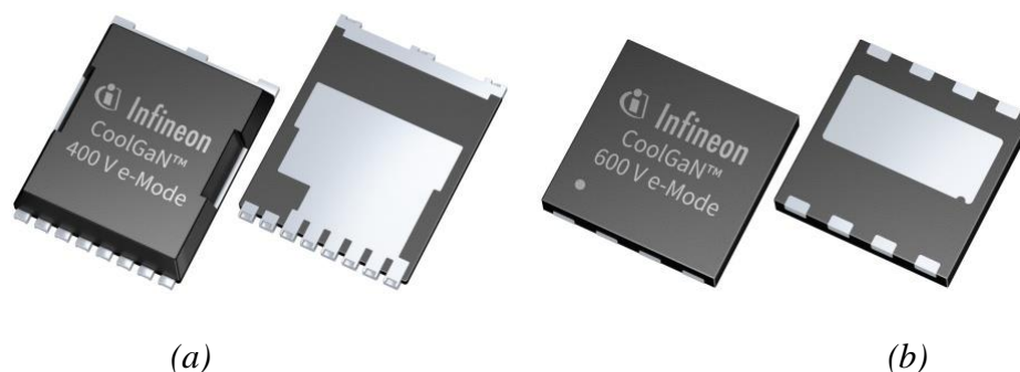
Figure. Targeting high end audio equipment, the IGT40R070D1 E8220 400-V GaN power transistor (a), enables smoother switching and a more linear class D output stage by offering low/linear C_{oss} , zero Q_{rr} , and a normally-off switch. The IGLD60R190D1, a 600-V 190-m \Omega , industrial-grade GaN HEMT (b) has been cost reduced for consumer and industrial applications.
