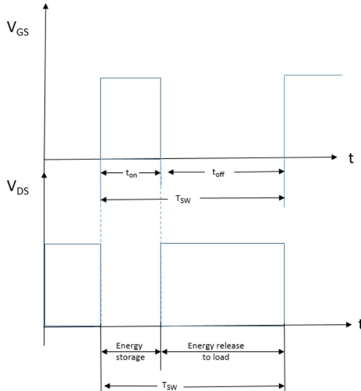
Fig. 1. Power switch waveforms contain the timing parameters needed to calculate core size for the distributed-gap inductor.
