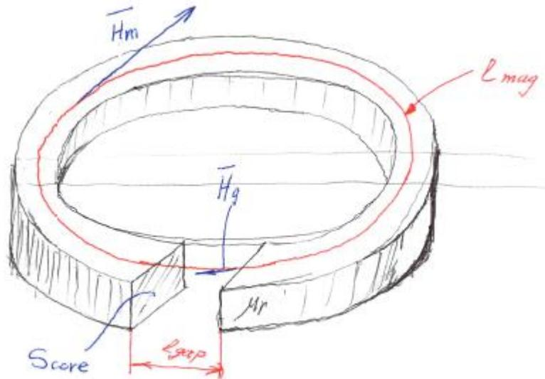
Fig. 2. Key parameters for calculating the size of the gap in a gapped-core ferrite inductor.
