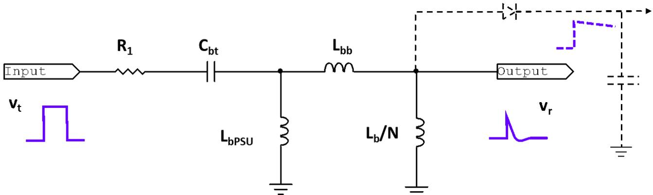
Fig. 4. An equivalent linear RLC circuit model can be used for analysis of transmission line voltage and current waveforms. The pulse duration at the receiver end can be extended with a peak detector having a needed hold time (dashed lines). For a version of the transmitter with transformer output, transformer leakage inductance needs to be added in series with  $R_1$ .
