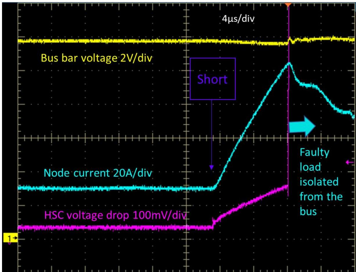
Fig. 6. With the selected 1-μH buffer inductor, the current ramped up in a controlled manner and at the time the HSC switch started isolating the faulty load from the power line, the short circuit current reached its maximum (105 A) while the power line voltage remained within its spec limits.
