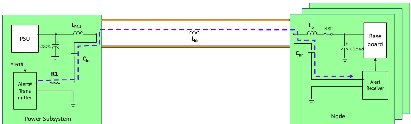
Fig. 3. Functional block diagram illustrating transmission of the alert signal across the dc power line.
