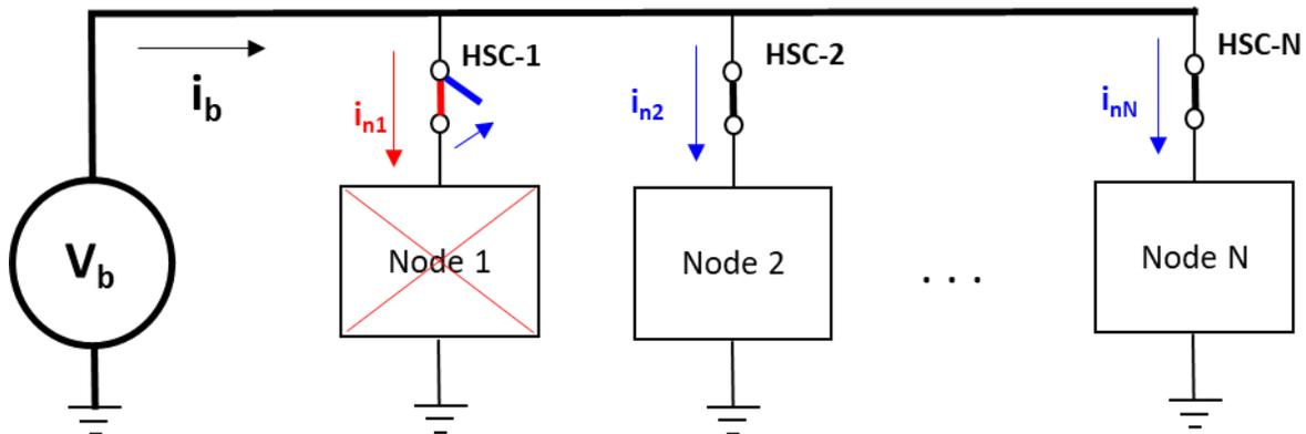
*Fig. 1. Simplified block-diagram of a common bus-bar dc PDN supplying power to N nodes. Protection of the PDN from node faults is provided with hot swap controllers detecting severe overcurrent and isolating the faulty load from the PDN. In absence of buffer inductors the current in the faulty node ( $i_{n1}$ ) and bus current  $i_b$  can reach excessive levels and even a very fast HSC response may not prevent excessive bus current and an out-of-spec condition for the bus voltage  $V_b$ .*
