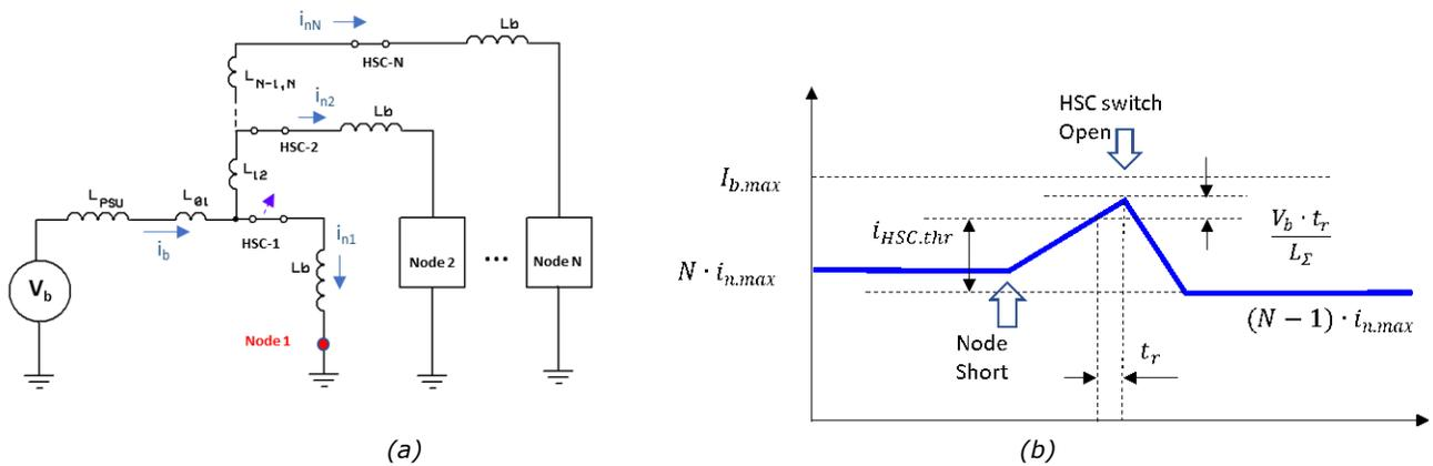
Fig. 2. Simplified equivalent circuit of a PDN delivering dc power to  $N$  nodes with node 1 failed into short circuit (a) and a PDN current diagram after a short circuit occurs in one of the nodes (b). The PDN current ramps up after a short and ramps down once the affected HSC switch isolates the faulty node from the bus.
