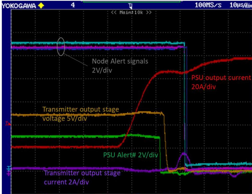
Fig. 7. In the overdamped mode only a single short current pulse is generated in the transmission line, which allows it to reliably generate alert signals in multiple receivers within a short (10- $\mu$ s) time interval.
