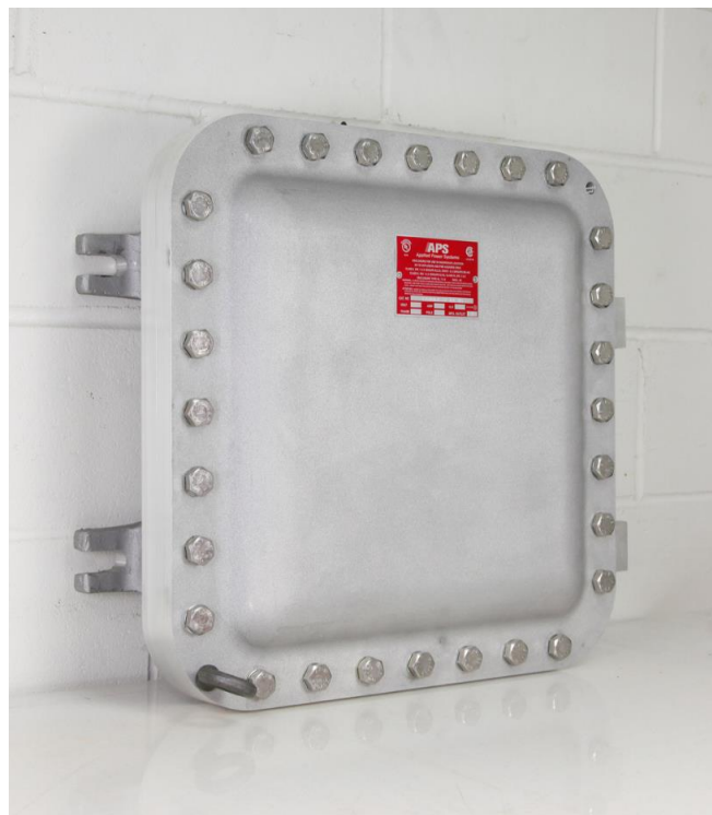
Figure. Housed in an aluminum explosion-proof enclosure, the BC-6494 battery charger can be factory programmed to support multiple battery stack configurations, ranging from 12 V at 100 A up to 72 V at 20 A charging power.
