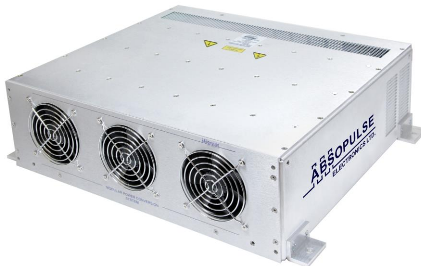
Figure. The HVI 5K-3U7 converters accept a 600-V nominal input voltage (or a 400-V to 800-V input range) and deliver up to 5-kW output at 24 V, 48 V, 110 V, 125 V or a custom value. A built-in redundancy diode allows paralleling of multiple converter units for higher power output or N+1 redundancy.
