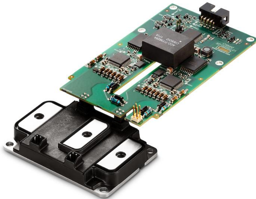
Figure. The CMT-TIT0697 gate driver board has been designed to be directly mounted on Wolfspeed's CAB450M12XM3 1200-V SiC MOSFET power modules. It safely drives the fast switching SiC power modules to achieve low losses while operating in high-temperature environments.
