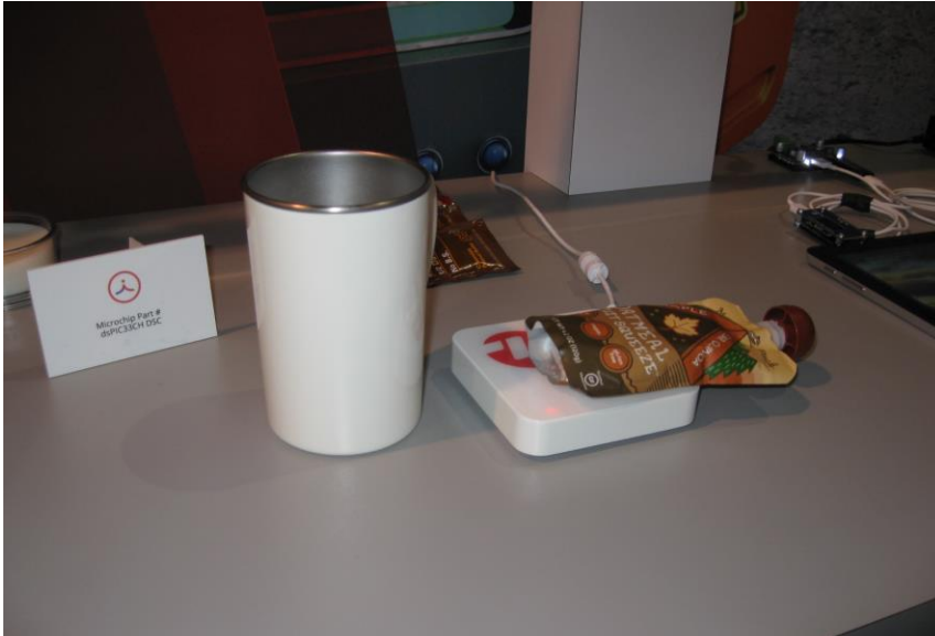
One of Microchip's dsPIC digital signal controllers is used in the design of a transmitter that performs both wireless charging of Qi-compliant devices and inductive heating of specially packaged foods.
