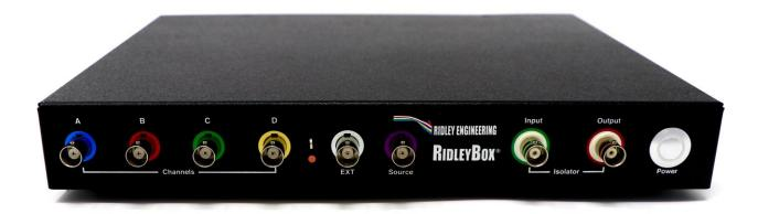
Figure. The RidleyBox combines a four-channel frequency response analyzer, a four-channel 200-MHz oscilloscope, a Ridley Universal Injector, and an Intel computer. A lifetime license for RidleyWorks Design Software is also included with this product.
