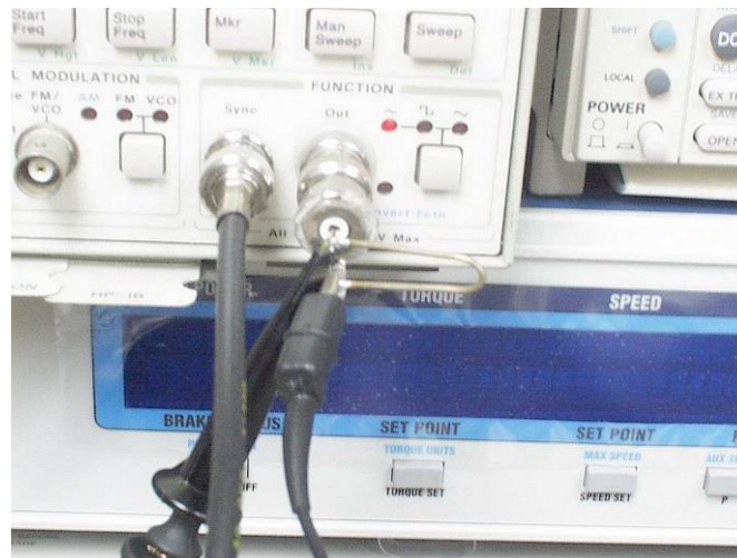
Fig. 6. The Fig. 4 test circuit constructed at the output of a function generator. The parallel half-loop of wire is the sense resistor. Although a \times 10 probe is sensing v_o , it is better to use a cable terminated in 50\ \Omega at the oscilloscope. For this circuit, R_g = 50\ \Omega , not 25\ \Omega , because it lacks a terminating 50\text{-}\Omega resistance.
