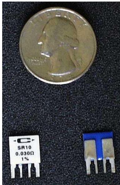
Fig. 3. Small metal-film resistors on a ceramic substrate (with a quarter shown for size). The outer terminals are the drive pair and the smaller inner terminals are for sensing voltage across the accurate 1% resistance.
