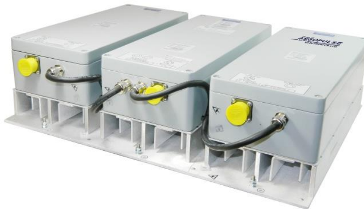
Figure. This high-frequency 1-kW PWM inverter converts 24-Vdc nominal input to 230-Vac continuous of pure sinewave output at 50 Hz. The inverter is built with three power modules in IP66 D3 size die cast aluminum enclosures. Two CDC 500 modules and one MSI 2300 module are used to generate the required output power. The dc-dc input stage boosts the input voltage to a higher dc voltage, which feeds the dc-ac inverter to generate the required ac output. The heatsink assembly and baseplate shown here provide pure convection cooling with additional cooling achieved by internal conduction to the walls of each enclosure, with additional convection via the outside surface.
