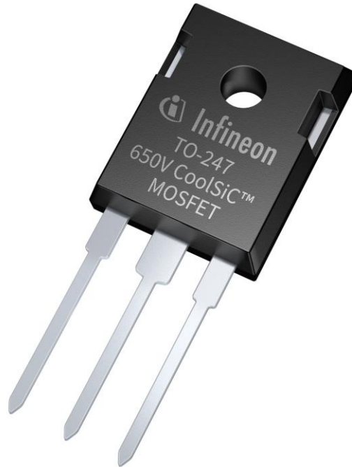
Figure. As with the 1200-V family members, the new 650-V CoolSiC MOSFETs are well suited for hard- and resonant-switching topologies such as LLC and ZVS, and can be driven like an IGBT or CoolMOS MOSFET, using standard drivers. According to Infineon, these robust devices offer superior gate-oxide reliability enabled by state-of-the-art trench design, best-in-class switching and conduction losses, highest transconductance level (gain), a 4-V threshold voltage and short-circuit robustness. These CoolSiC MOSFET 650-V devices are rated from 27 mΩ to 107 mΩ.
