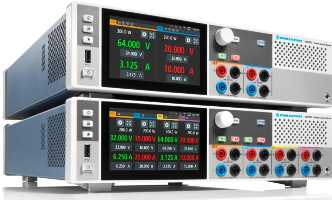
Figure. The five R&S NGP800 models meet the needs of users seeking minimum device footprint for two or four independent power supplies, with maximum flexibility for voltages up to 250 V, currents up to 80 A and power up to 800 W. Each channel supplies up to 200 W with a maximum of 20 A or 64 V, also covering 48-V automotive and industrial applications.
