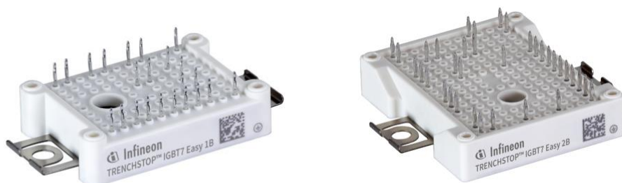
Figure. Based on the new micro-pattern trench technology, the TRENCHSTOP IGBT7 chips of the Easy 1B/2B portfolio have much lower static losses compared to the IGBT4 chips with the on-state voltage reduced by 20%.
