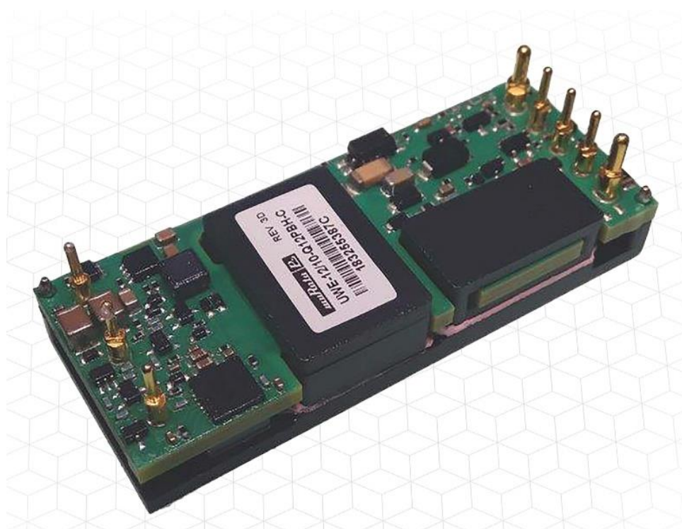
Figure. Operating from a 9- to 36-V input range suitable for industrial applications, the UWE-Q12 series isolated dc-dc converters in the eighth-brick format generate a fully regulated output of 5 V, 12 V, or 24 V, all rated at 120 W.
