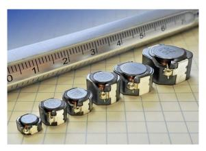
performance are superior to other similar-size devices in the market, according to the vendor. At the same time, the ferrite drum and ring core architecture is said to offer very effective magnetic shielding. As automotive circuit densities increase, the effectiveness of this shielding grows in importance, in order to minimize EMI that could interfere with adjacent circuitry.
