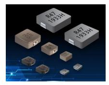
The SRP1040VA and SRP6030VA inductors are built with a new metal alloy powder formulation and round enamel-coated copper wire. The company's innovative metal alloy powder formulation allows an elevated operating temperature of 180°C (including self-heating). This makes these AEC-Q200 compliant inductors well suited for many high-temperature environments and high-reliability designs including LED lighting, dc-dc converters and power supplies. Inductance values range from 0.47 to 22  $\mu$ H.
