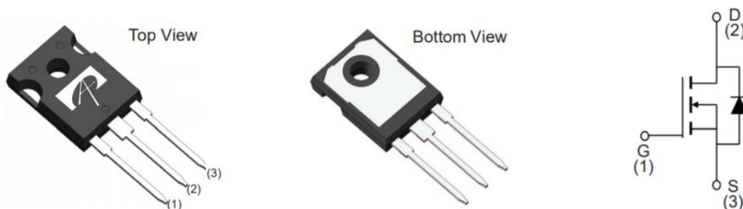
Figure. The low internal resistance of the AOK065V120X2 1200-V SiC MOSFET enables fast switching and low loss. The transistor is designed to be driven with a -5-V/+15-V gate drive, allowing the broadest compatibility with existing high-voltage IGBT and SiC gate drivers.
