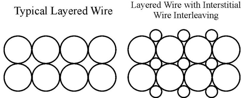
Fig. 1. Comparison of ordinary layered wire in a winding (left) and the same winding with additional, interstitial wire (right) that increases the winding packing factor.
