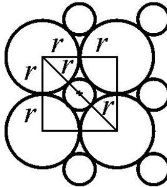
Fig. 2. Closer view of winding with square constructed on the adjacent wire centers of wire of radius,  $r$ .
