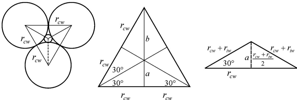
Fig. 3. Interstitial wire between layers of round wire of the hexagonal layer configuration (left); the triangle, inverted and bisected (center); and the lower triangle detail (right).
