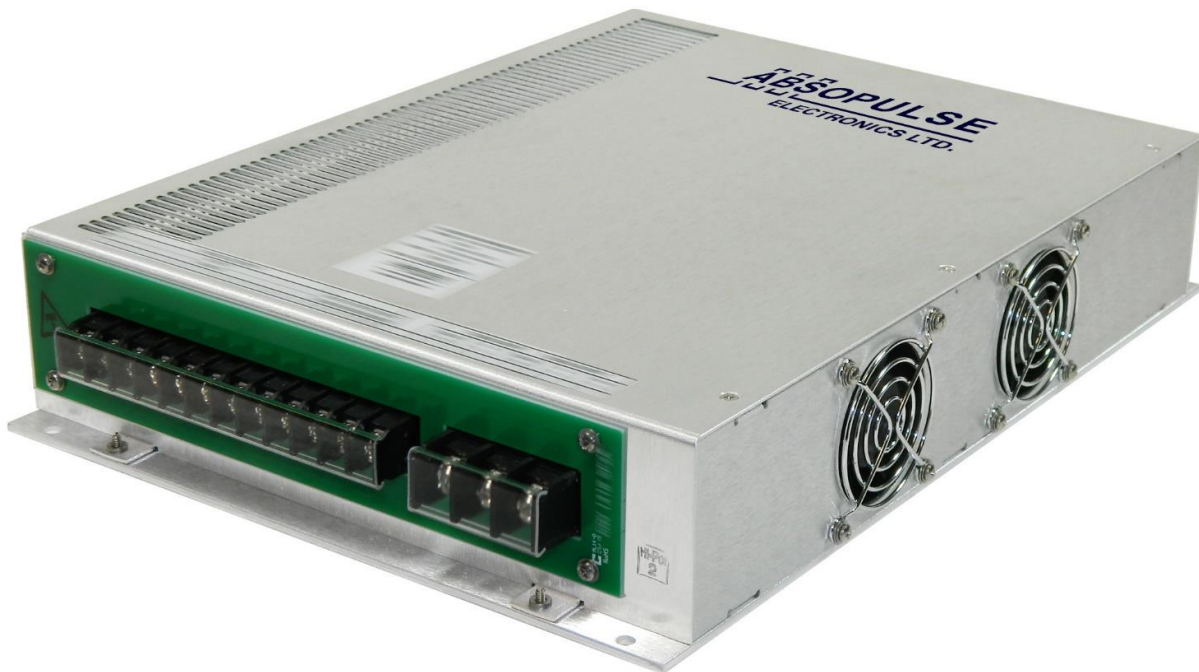
Figure. The PFL 2K-E/110-F6W is a 2-kW switching power supply with power factor correction (PFC), rugged industrial quality, a field-proven design topology, full electronic protection and N+1 redundancy as an option. The unit measures 254 x 65 x 349 mm (10 x 2.6 x 13.75 in.) including mounting flanges and terminal block, and weighs 3.3 kg (7.5 lbs).
