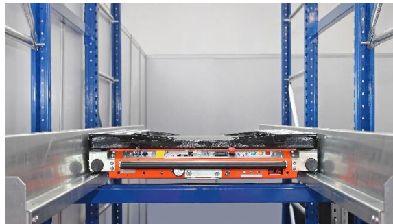
Fig. 1. Centered on the rails is a typical motorized pallet shuttle. (Transfer car is not pictured.)
