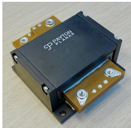
Figure. Payton says its 10-kW planar transformer is the first high-voltage planar transformer with a partial discharge extinction voltage (<10 pC) of 10 kV between primary, secondary and core. Because partial discharges in a transformer deteriorate its insulation and can lead to failure of the transformer, they degrade its long-term reliability. By addressing this problem, Payton can satisfy the demands of critical applications requiring 20+ years of operation.
