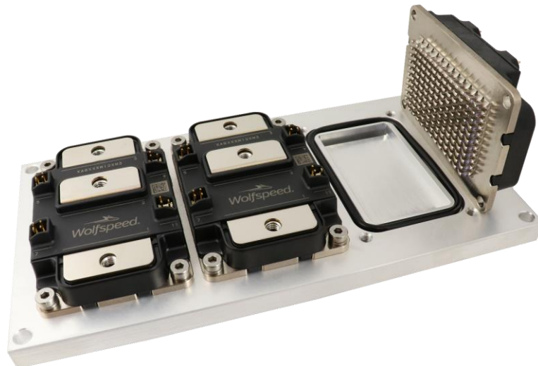
Fig. 6. Assembly of direct-cooled XM3 modules mounted on a cold plate as used in the test setup with one position removed to show the coolant chamber and gasket.
