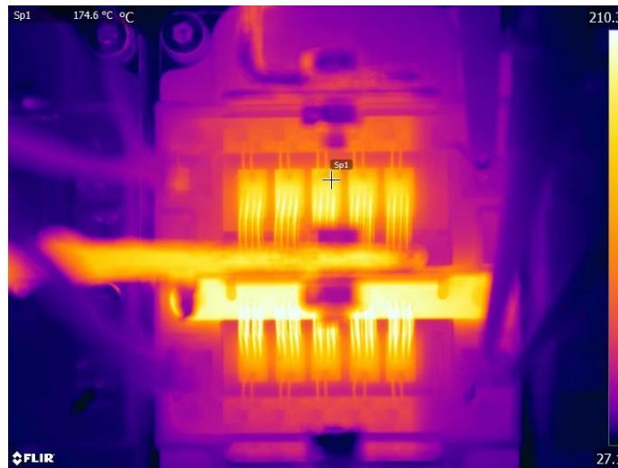
Fig. 7. Thermal image of an open module painted black.
