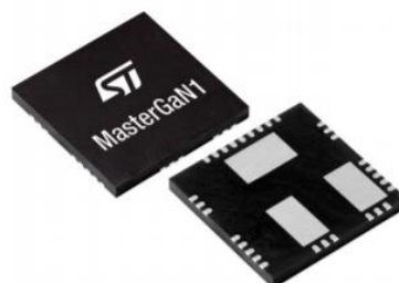
Figure. The MASTERGAN1 is a power system-in-package co-packaging a gate driver and two 650-V 150-mΩ enhancement-mode GaN HEMT transistors in half-bridge configuration with integrated bootstrap diode and UVLO protection on both the lower and upper driving sections. The device is housed in a compact 9-mm x 9-mm QFN package as shown on the right.
