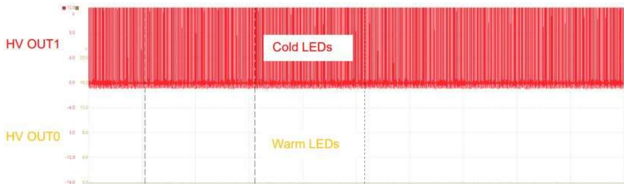
Fig. 11. Cold LEDs on max brightness. Current goes from HV OUT1 to HV OUT0 through the cold LED string only.
