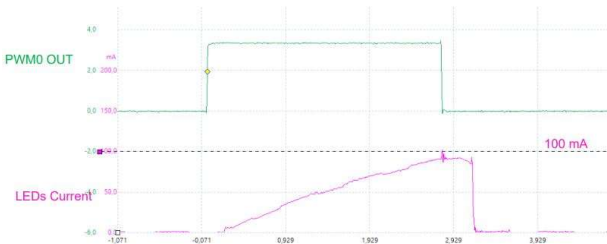
Fig 9. Current limitation. When LED current exceeds the 100-mA threshold, the PWM0 output, which controls brightness, goes low.
