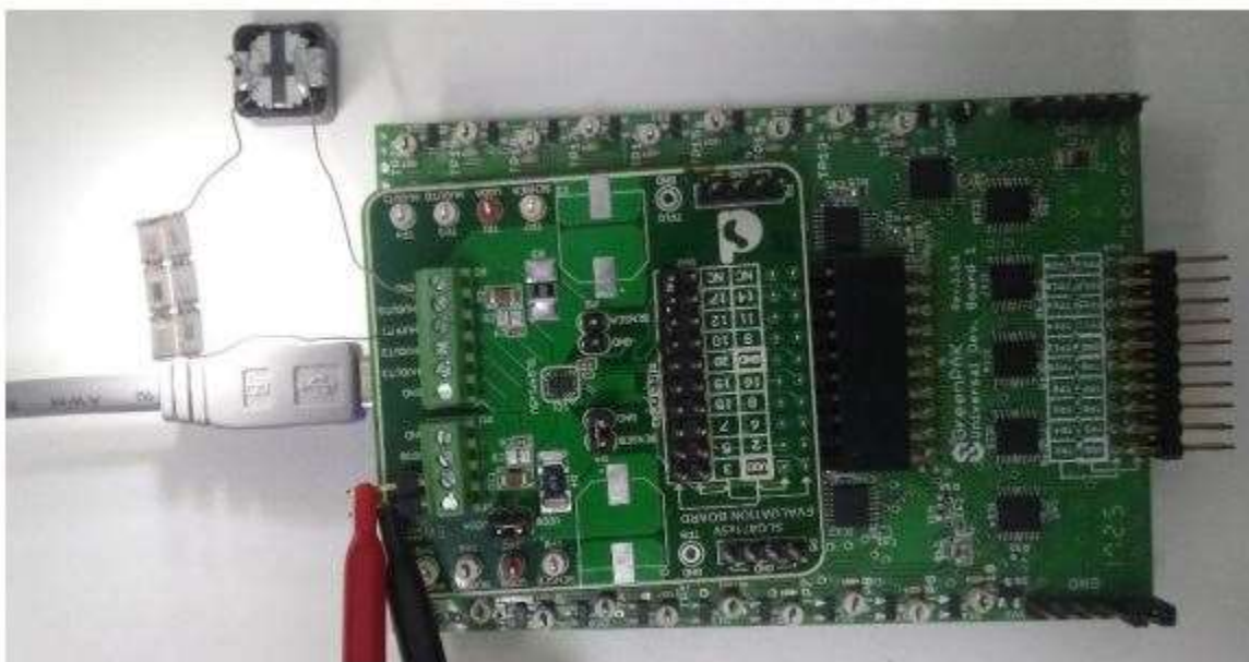
Fig. 5. The same LED driver circuit operated with buttons set for cold LEDs on and warm LEDs off. The cold LEDs produce a whiter light.
