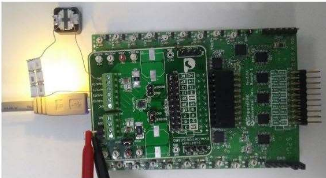
Fig. 4. The HV PAK eval board configured with the proposed LED driver design, operated with buttons set for warm LEDs on and cold LEDs off. The warm LEDs produce a yellowish light.
