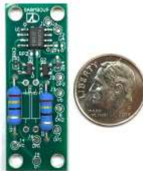
Figure. ALD's SABMBOVP2XX family of overvoltage protection printed circuit boards consists of innovative circuits designed to provide precision overvoltage protection in stacked supercapacitor voltage balancing and other voltage clamping applications. The SABMBOVP2XX circuit can be viewed as a precision voltage clamp circuit that offers a superior zener-diode type of functionality and performs to superior specification and characteristics in creating a strong, precision voltage clamp. Typically, the clamp current changes from a few nanoamps to over 100 mA at the clamp voltage within a 100-mV transition.
