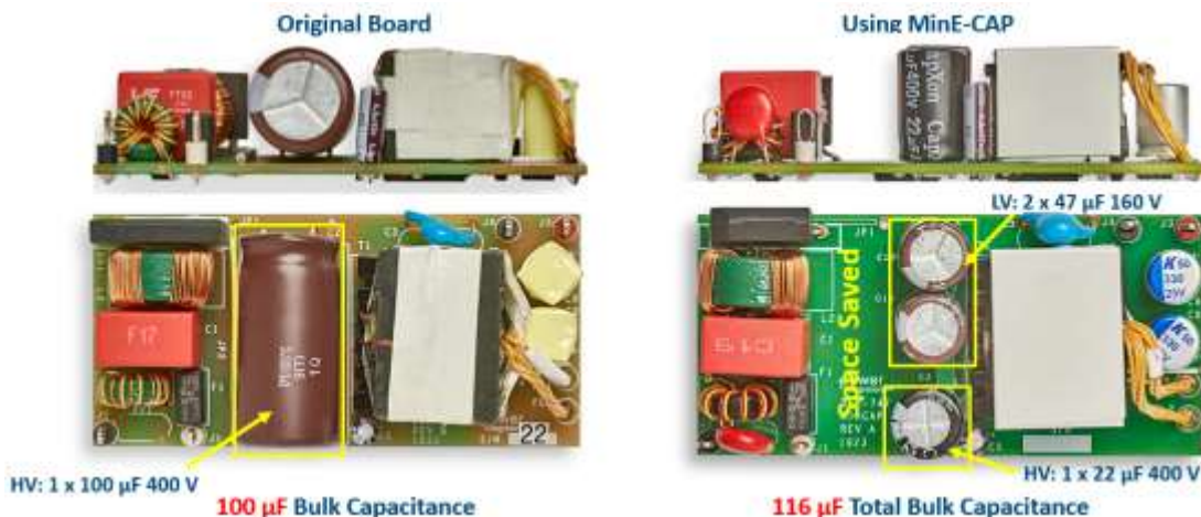
Fig. 2. In this example power supply design, MinE-CAP, replaces one 400-V 100- \mu F bulk capacitor with one 400-V 22- \mu F capacitor and two 160-V 47- \mu F capacitors, saving space as illustrated here. In addition to reducing the total volume of the capacitors required for bulk energy storage by 50%, this technique reduces inrush current and increases the total capacitance by 16%, enabling more peak power.
