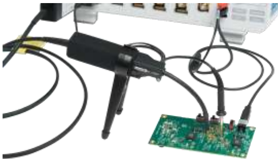
Fig. 1. Like the first generation, the IsoVu Gen 2 probes use patented electro-optical technologies to capture signals and power the probes without the need for an electrical connection to the oscilloscope. They offer a unique combination of high bandwidth, dynamic range and CMRR over the probe's full bandwidth. But these second-gen IsoVu probes also offer greater robustness, higher bandwidth, smaller size and lower cost than their predecessors.
