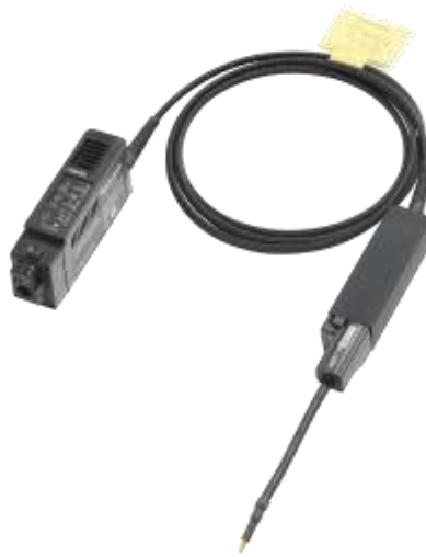
Fig. 1. Like the first generation, the IsoVu Gen 2 probes use patented electro-optical technologies to capture signals and power the probes without the need for an electrical connection to the oscilloscope. They offer a unique combination of high bandwidth, dynamic range and CMRR over the probe's full bandwidth. But these second-gen IsoVu probes also offer greater robustness, higher bandwidth, smaller size and lower cost than their predecessors.
