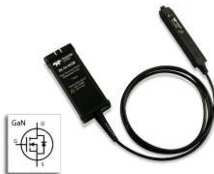
Figure. 60 V of common mode and 80 V of differential input range with up to 1-GHz bandwidth make the DL-HCM probe series well suited for lower-voltage GaN power conversion measurements. They feature 0.5% dc gain accuracy for high-precision measurements, 0.1-dB flatness from dc to 100 MHz, exceptional CMRR out to very high frequencies, 50 dB at 100 MHz, a wide variety of tips that come standard, and an optional accessory kit.
