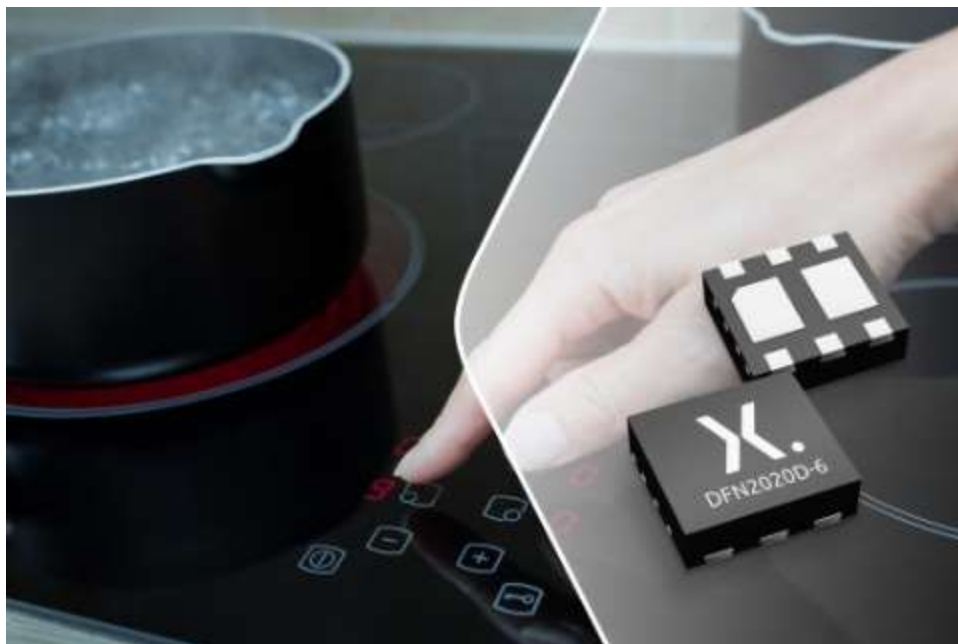
Figure. The AEC-Q101-qualified DFN2020D-6 LED driver ICs save up to 90% PCB space, while also featuring side-wettable flanks that enable automated inspection and improve reliability.
