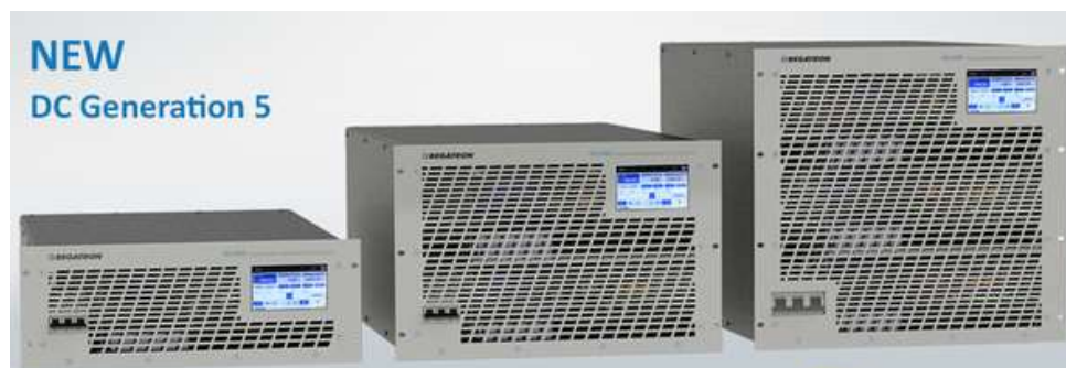
Figure. Suitable for a wide range of industrial and scientific applications, REGATRON's DC Generation 5 programmable regenerative dc power supplies are technologically advanced, fast switching, compact 19-inch power supplies that feature control dynamics in the 100- to 200- \mu s range, even at higher power levels. They also exhibit exceptional current accuracy of <0.02% full scale, with additional high-resolution current measurement range. The power output capability of an individual power supply ranges from 0 to 18 kW up to 0 to 2000+ kW, with output voltage up to 3000 Vdc.
