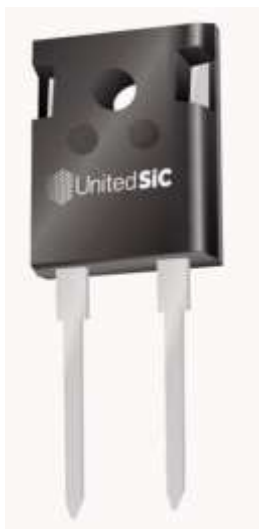
Figure. The third-generation SiC merged-PiN-Schottky (MPS) diodes, which offer current ratings of 25 A at a 1700-V blocking voltage, and 10 A, 20 A or 50 A at a 1200-V blocking voltage, are said to offer the industry's best surge current performance. For example, the 10-A 1200-V SiC Schottky specifies a non-repetitive forward surge current sine half wave rating of 120 A at 25°C.
